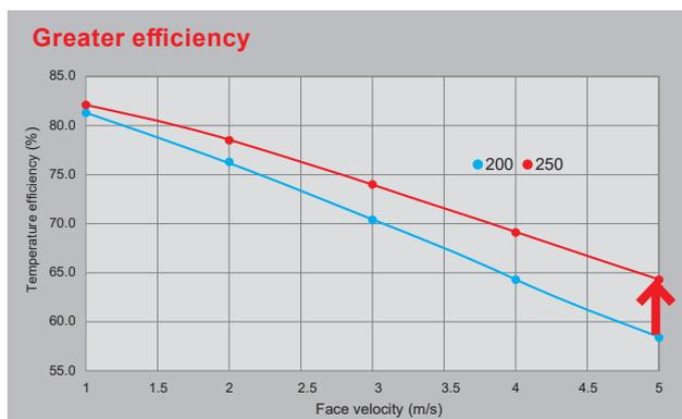
Significantly increased heat recovery efficiency in the case of the 250 mm series (red) in comparison to the standard design.
