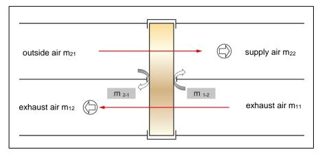
Figure 4: Outside air fan sucks in - exhaust air fan sucks in
