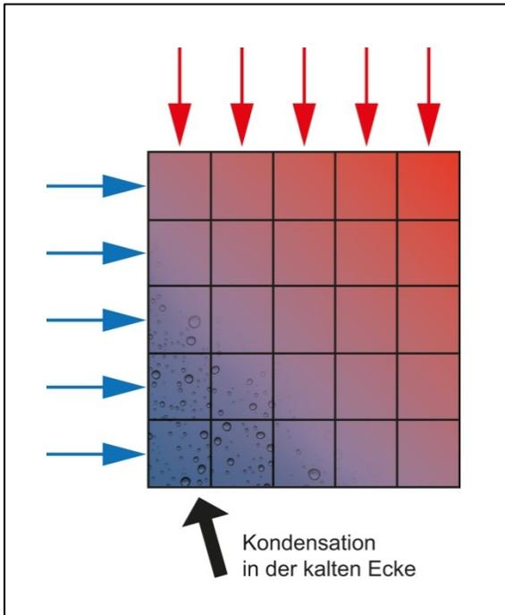
Figure 2: Condensation first occurs in the "cold corner"
