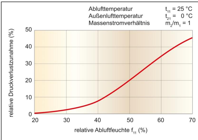
Diagram 2: Pressure loss increase with condensation
